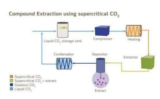
Figure 3.3: Supercritical carbon dioxide extraction
